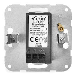
Mounting: built-in (clamp and / or screw) Diameter including matrix: 71x78x42 mm Product weight: 85 grams Installation depth: 26 mm Suitable for existing flush-mounted boxes
